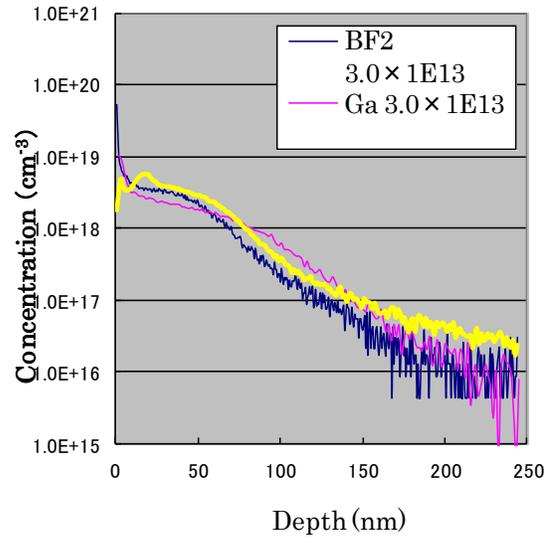
**FIGURE 2.** SIMS profiles after annealing
