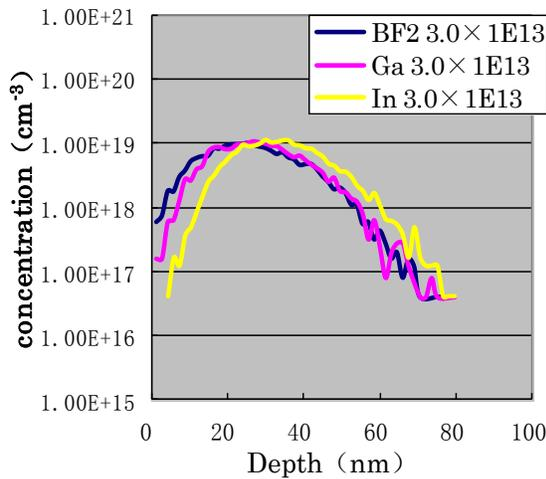
**FIGURE 1.** As-implanted profiles obtained by TRIM simulation
