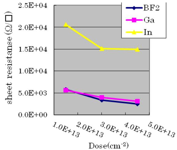
**FIGURE 5.** Sheet resistance ( $R_s$ ) as a function of implanted doses
