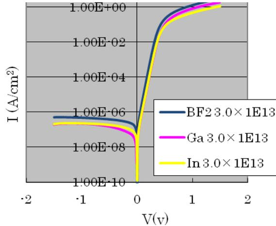
Figure 6. Diode I-V characteristics
