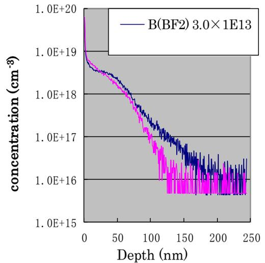
**FIGURE 3.** SIMS profiles of BF<sub>2</sub> and In + BF<sub>2</sub>
