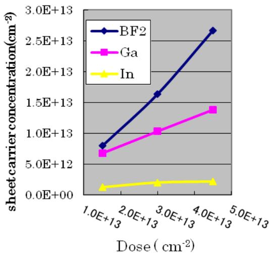
**Figure 4.** Sheet carrier concentration as a function of implanted doses
