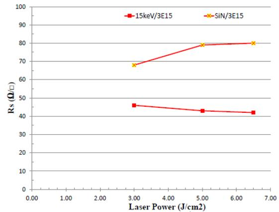
Fig.18: 15keV B-implant at 3E15/cm<sup>2</sup> dose Rs results comparing various laser annealing conditions either before or after SiN/ARC.
