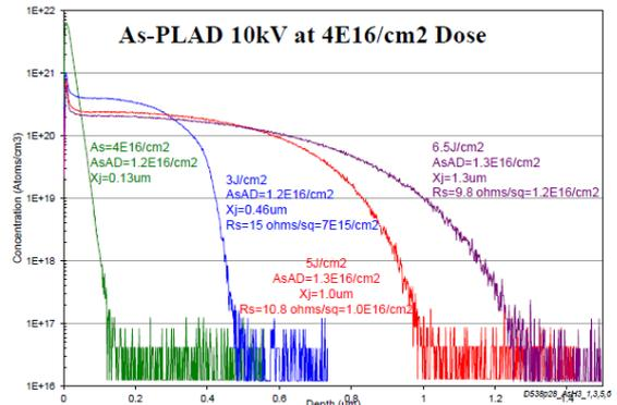
Fig.10: 10kV As-plasma implant at  $4E16/cm^2$  dose SIMS areal density analysis.
