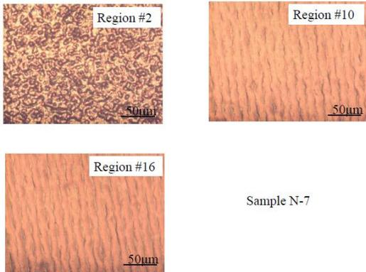
Fig.16: Optical micrographs of 3.0, 5.0 and 6.5 J/cm<sup>2</sup> laser annealed regions showing SiN removal and melted silicon textured surface from Fig.5.
