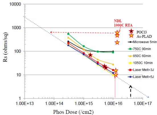
Fig.7: Rs versus 15keV P-implant dose for various annealing methods.
