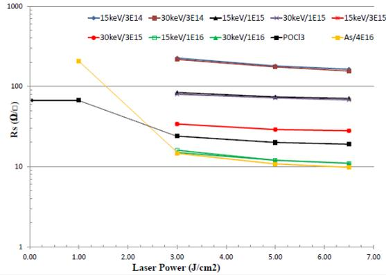
Fig.6: POCl<sub>3</sub>, phosphorus and arsenic implant Rs results at various laser power conditions.
