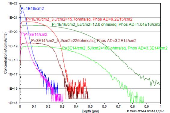
Fig.9: P-implant at 15keV  $3E14/cm^2$  and  $1E16/cm^2$  dose P-SIMS areal density analysis.
