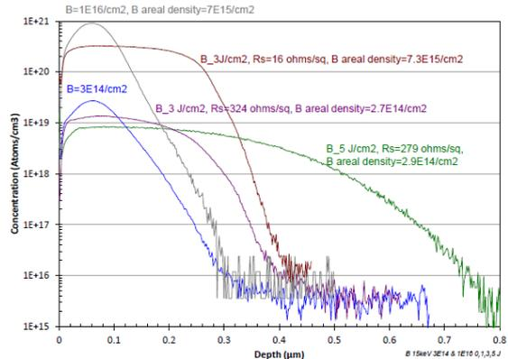
Fig.14:  $15\text{keV}$  B-implant at  $3\text{E}14/\text{cm}^2$  and  $1\text{E}16/\text{cm}^2$  dose B-SIMS areal density analysis.
