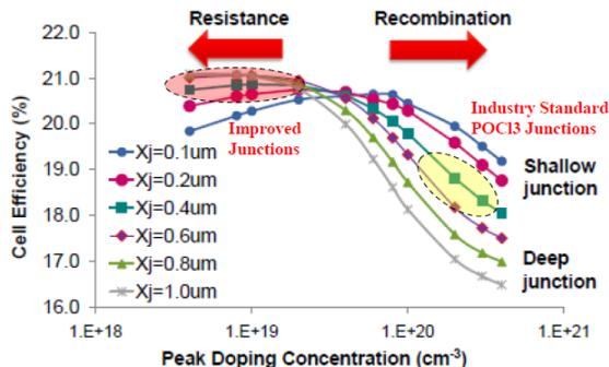
Fig.1: Simulation results for cell efficiency based on surface doping concentration [1].
