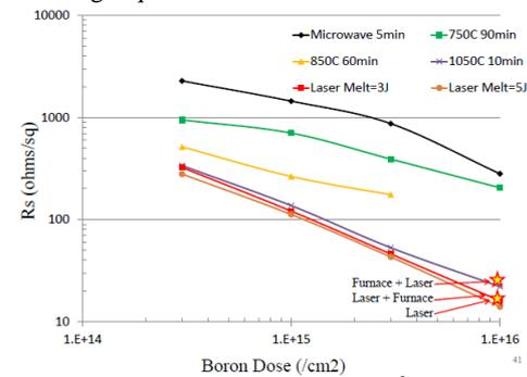
Fig.29: B-implant 15keV at  $1E16/cm^2$  dose  $R_s$  results for laser, laser + furnace and furnace + laser annealing sequences.
