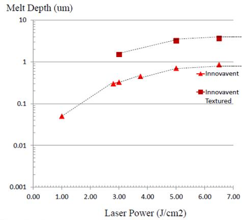
Fig.23: Silicon melt depth versus laser power for polished and textured silicon surfaces.
