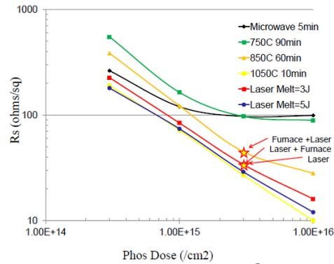
Fig.28: P-implant 15keV at  $3E15/cm^2$  dose  $R_s$  results for laser, laser + post-furnace and pre-furnace + laser annealing sequences.
