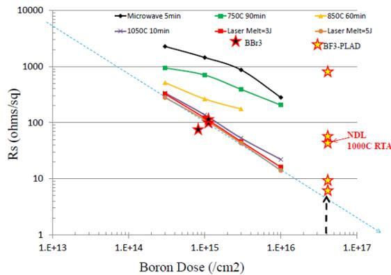
Fig.12:  $R_s$  versus  $15\text{keV}$  B-implant dose for various annealing methods.
