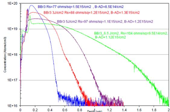
Fig.13:  $\text{BBr}_3$   $11\text{B}$ -SIMS areal density analysis.
