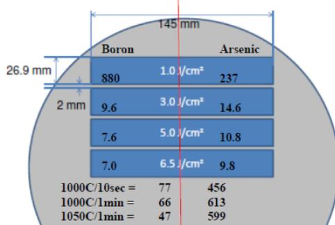
Fig.3: Plasma implant wafer laser annealing pattern.
