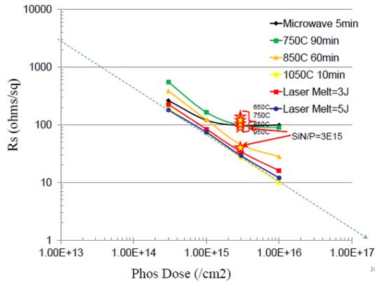
Fig.24: SiN/P-implant Rs versus RTA annealing temperature.
