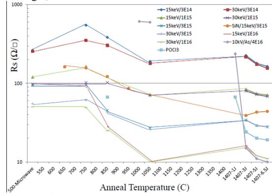
Fig.26: N-type P and As dopant  $R_s$  versus annealing temperature condition.
