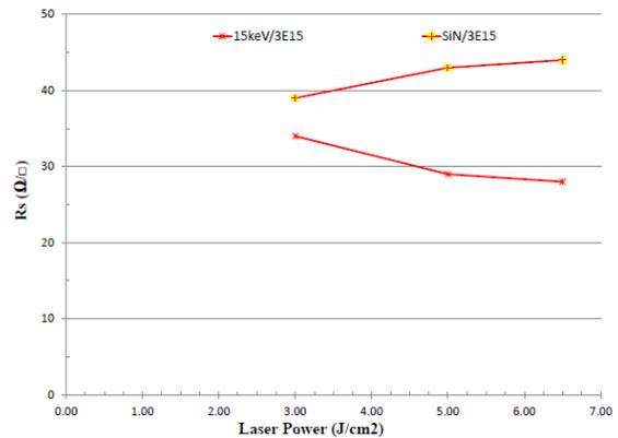
Fig.17: 15keV P-implant at 3E15/cm<sup>2</sup> dose Rs results comparing various laser annealing conditions either before or after SiN/ARC.
