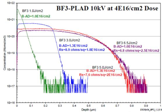
Fig.15: 10kV BF<sub>3</sub>-plasma implant at 4E16/cm<sup>2</sup> dose 11B-SIMS areal density analysis.
