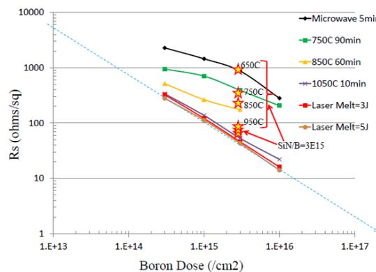
Fig.25: SiN/B-implant Rs versus RTA annealing temperature.
