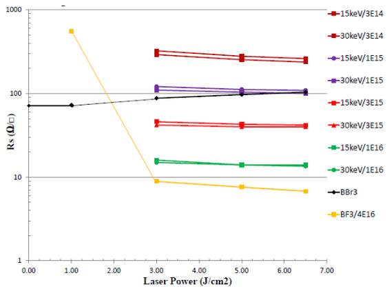
Fig.11:  $\text{BBr}_3$ , B and  $\text{BF}_3$  implant  $R_s$  results at various laser power conditions.
