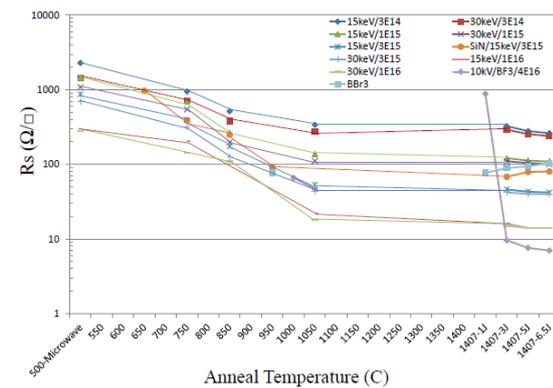
Fig.27: B dopant  $R_s$  versus annealing temperature condition.
