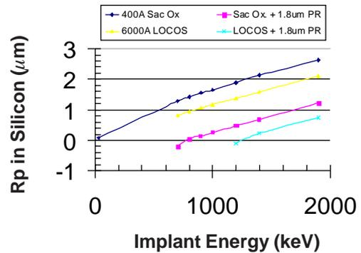
Fig 3. Boron implant profiles for BILLI processing
