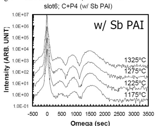
Fig.13c: HR-XRD for C+P<sub>4</sub> with Sb-PAI.
