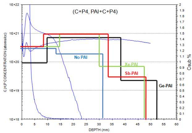
Fig. 17b: Csub modeling for C+P<sub>4</sub> and PAI+C+P<sub>4</sub>.
