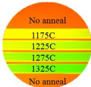
Fig.5: TW full wafer image showing the 4 different laser annealing temperature regions and no anneal regions.
