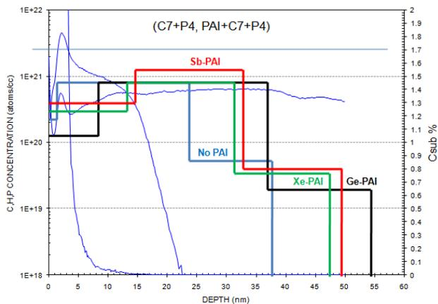
Fig. 17c: Csub modeling for C<sub>7</sub>+P<sub>4</sub> and PAI+C<sub>7</sub>+P<sub>4</sub>.
