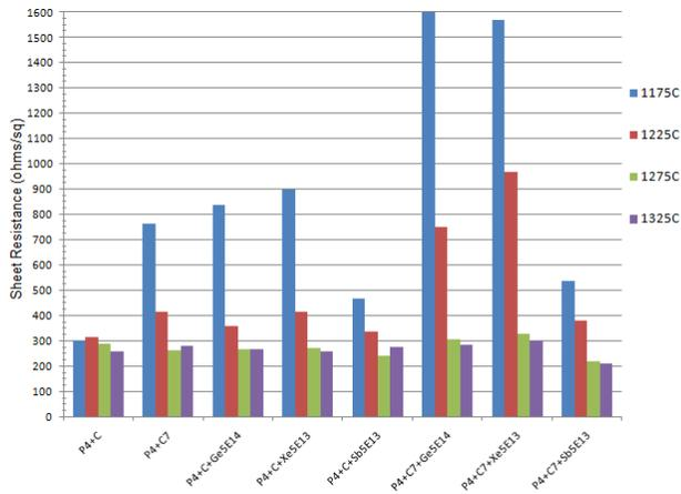
Fig.8: Sheet resistance (Rs) results.
