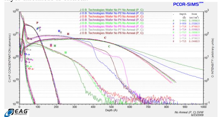
Fig.6: P & C PCOR-SIMS depth profiles in the no anneal region.
