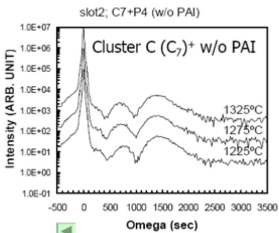
Fig.12b: HR-XRD rocking curve for C<sub>7</sub>+P<sub>4</sub>.
