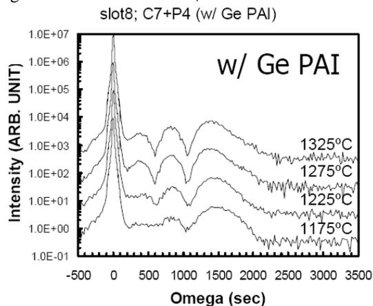
Fig.14a: HR-XRD for C<sub>7</sub>+P<sub>4</sub> with Ge-PAI.
