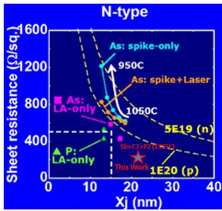
Fig.9: Rs versus Xj chart showing Pss~4E20/cm<sup>3</sup>.
