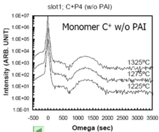
Fig.12a: HR-XRD rocking curve for C+P<sub>4</sub>.
