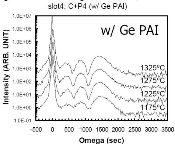
Fig.13a: HR-XRD for C+P<sub>4</sub> with Ge-PAI.
