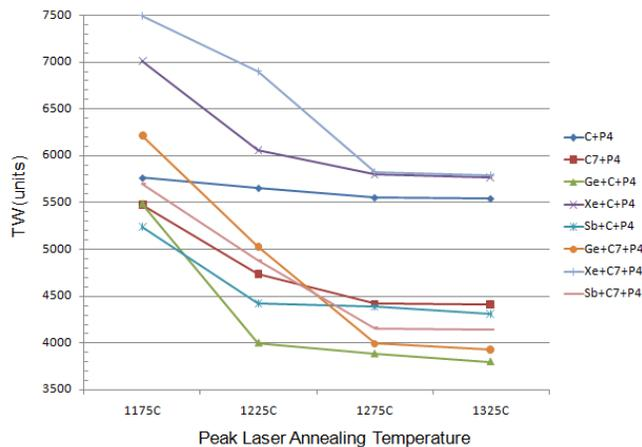
Fig.10: TW results to detect the level of residual implant damage after the various anneals.
