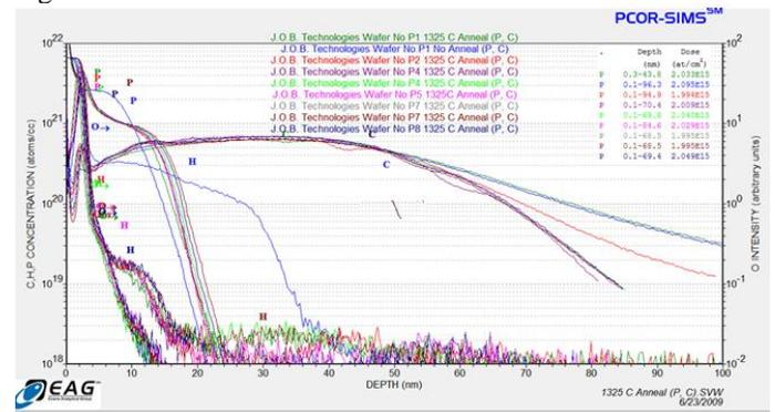
Fig.7: P & C PCOR-SIMS depth profiles in the 1325°C anneal region.
