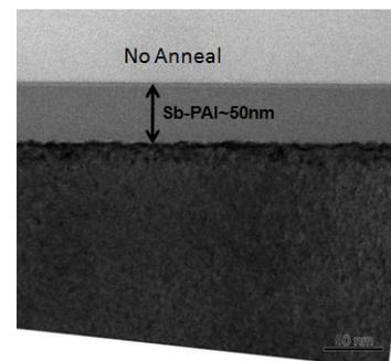
Fig.2: X-TEM of Sb-PAI no anneal region showing 50nm deep amorphous layer for 60keV/5E13/cm<sup>2</sup> implant.
