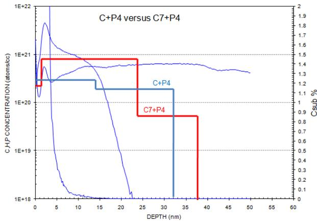
Fig. 17a: Csub depth modeling for C+P<sub>4</sub> versus C<sub>7</sub>+P<sub>4</sub>.
