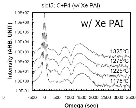
Fig.13b: HR-XRD for C+P<sub>4</sub> with Xe-PAI.
