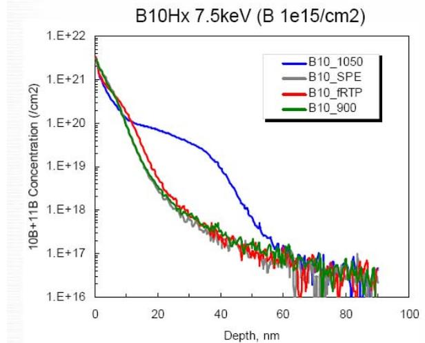
Fig.12: Diffusion-less spike annealing at 900°C [15].
