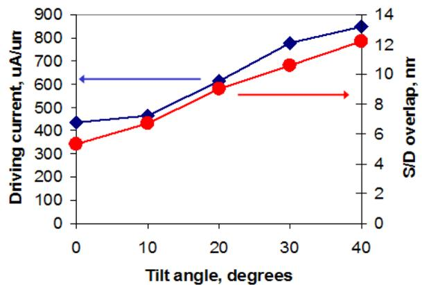
Fig.7: Arsenic tilted extension implantation for improved gate overlap control [11].
