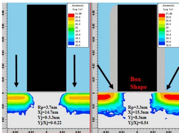
Fig.5: Arsenic 0 and 30 degree tilt implant showing little lateral straggle [10].
