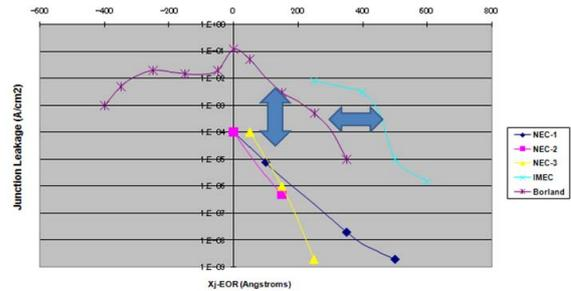
Fig.2: Different diode junction leakage current results for various PAI EOR damage depths [1,2,3].
