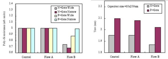
Fig.11: Comparison of gate poly for msec+spike (flow A) or spike+msec (flow B) [14].
