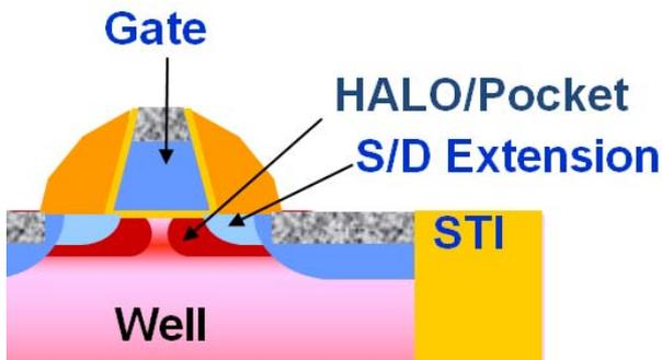
Fig.13: Gate leakage, S/D leakage or SDE/HALO gate edge leakage (band to band tunneling).
