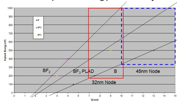
Fig.3: Boron extension implant energies without dopant channeling [4].
