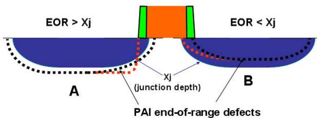
Fig.1: Location of EOR damage on junction quality [1].
