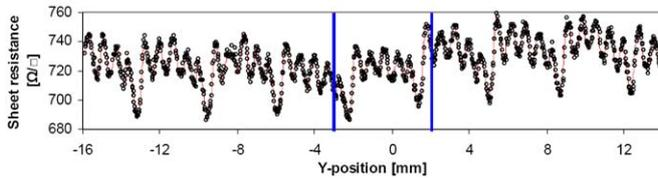
Fig.9: Rs micro-variation caused by laser annealing [13].
