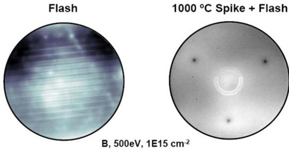
Fig.8: Therma-probe full wafer images comparing Flash only to spike+Flash annealing combination.
