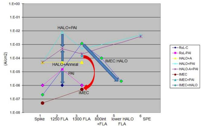
Fig.15: Effects of annealing on junction leakage.
