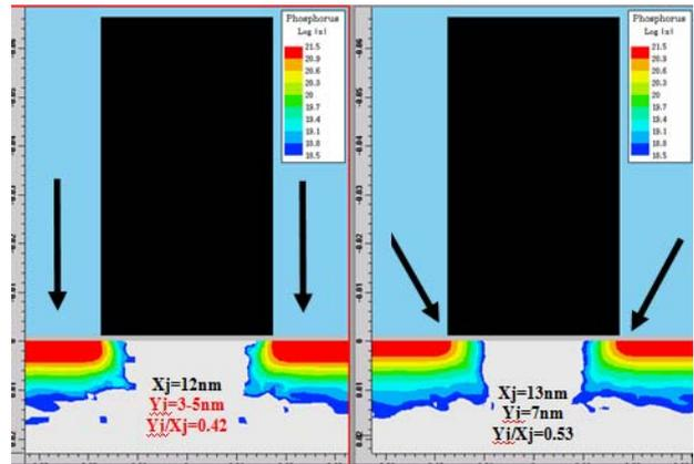
Fig.6: Phosphorus 0 and 30 degree tilt implant showing significant lateral straggle.
