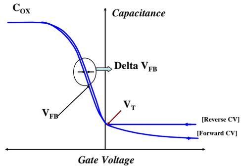
**FIGURE 2.** General CV curves depicting the non-equilibrium and equilibrium CV regions. The Forward sweep CV data represent non-equilibrium and the Reverse sweep CV data represent equilibrium CV data. Generally a light is used to generate carriers and form a surface inversion layer.
