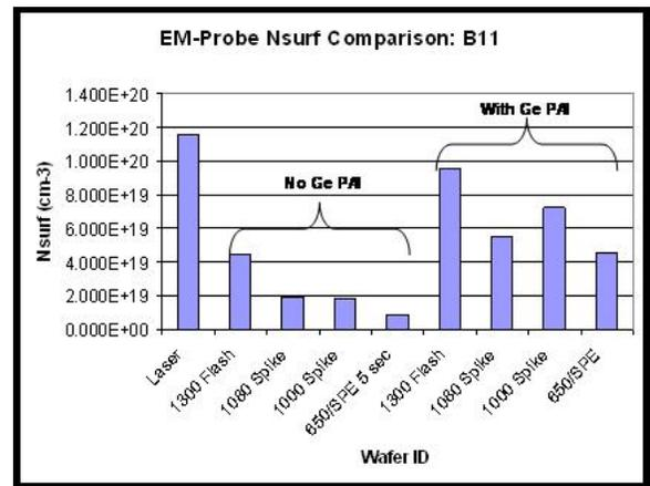
**FIGURE 3.**  $N_{SURF}$  results for B<sub>11</sub> S/D Implant with the five anneals shown and with and without PAI. The measured  $N_{SURF}$  values in each case match the expected activation levels.
