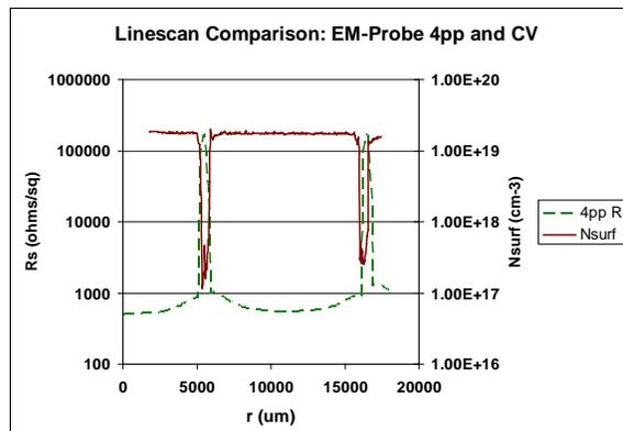
**FIGURE 5.** EM-Probe CV and 4pp  $R_S$  radial scans made on a laser annealed wafer piece.
