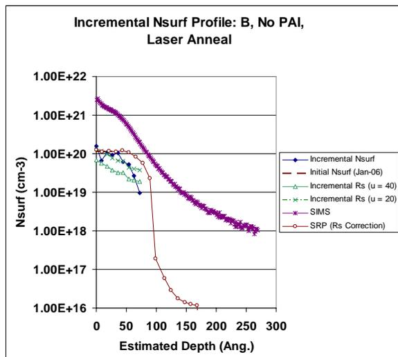
**FIGURE 4.** Profile Comparison: SIMS, SRP, Incremental CV ( $N_{SURF}$ ) and Incremental 4pp  $R_S$ .
