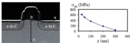
**Figure 5.** Cross-sectional STEM image (left) of an NFET with e-Si:C before silicidation, and (right) the uniaxial tensile stress ( $\sigma_{xx}$ ) measured by CBED as a function of depth ( $z$ ) at the center of the channel ( $x = 0$ ). The stress at  $z = 25\text{nm}$  is 615 MPa.
