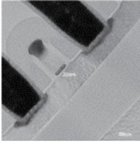
**Figure 4.** TEM image of the HK/MG nFET at 32nm L gate.
