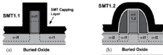
**Figure 6.** AMD reported using just a pre-amorphization implant with either the nSDE (n-type source/drain extension) or a deep n+S/D followed by a low-temperature solid phase epitaxy in the temperature range of 580–850°C.
