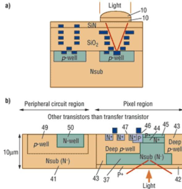
Figure 2. a) Metal layout above the photodiode maximizes light transmittance for frontside illumination in comparison to backside illumination. b) A deep n-well under the photodiode increases the light-sensitive area for backside illumination [6].
