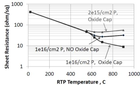
Fig.4. P Rs versus RTA temperature for 2E15/cm<sup>2</sup> and 1E16/cm<sup>2</sup> dose and without oxide surface capping layer.
