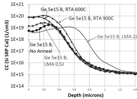
Fig.3. SRP of B 5E15/cm<sup>2</sup> after RTA annealing and laser melt annealing.
