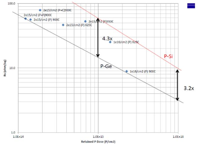
Fig. 8. Corrected  $R_s$  versus P-retained dose in Ge.
