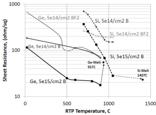
Fig.1. 4PP Rs versus anneal temperature for B and BF<sub>2</sub> implants.
