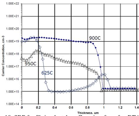
Fig.10. SRP for Sb-implant 1um Ge-epi wafers after RTA annealing.
