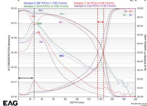
Fig.5: SIMS elemental concentration depth profile for 550°C RTA anneal cases.
