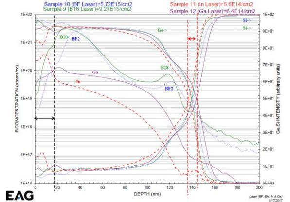
Fig.8: SIMS elemental concentration depth profile for laser annealed cases.
