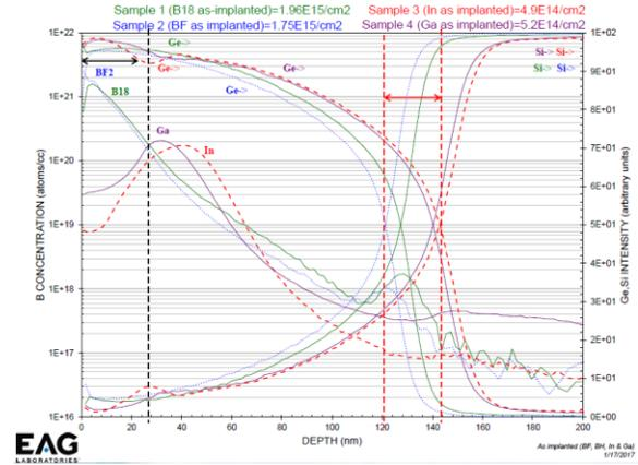
Fig.2: SIMS elemental concentration depth profile for as implanted no anneal cases.
