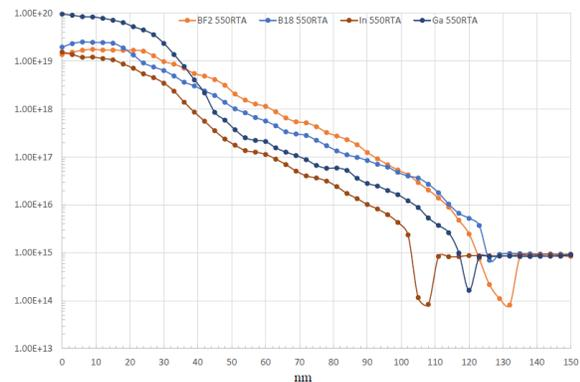
Fig.6: SRP electrically active carrier density depth profile for 550°C RTA anneal cases.
