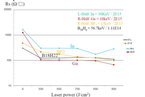
Fig.1: Rs 4PP results for as implanted no anneal and RTA/10sec at 550°C, 650°C, 750°C, 850°C and 950°C.
