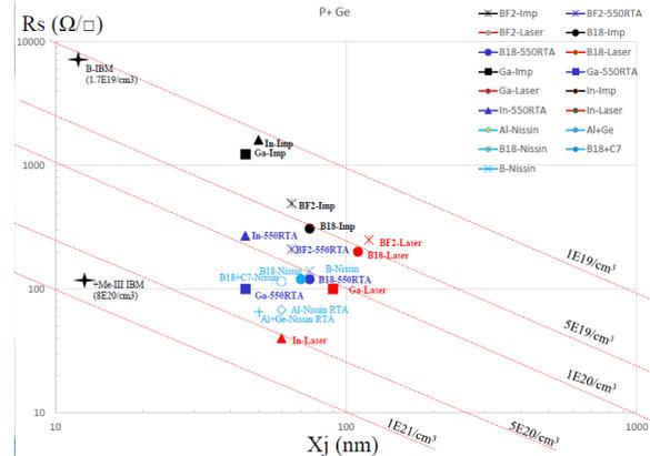
Fig.3: Rs versus X<sub>j</sub> plot for p+ doping in Ge.
