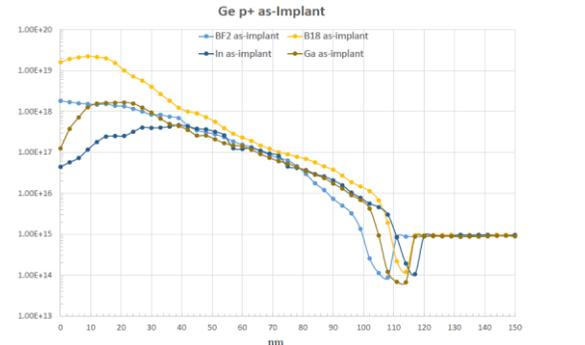
Fig.4: SRP electrically active carrier density depth profile for as implanted no anneal cases.
