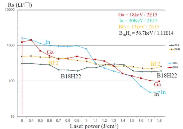
Fig.7: Rs 4PP results for 308nm laser anneal.
