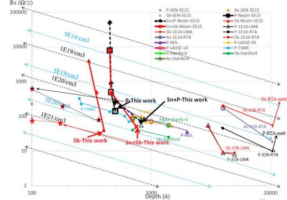
Fig.10:  $R_s$  sheet resistance versus n+ junction depth.
