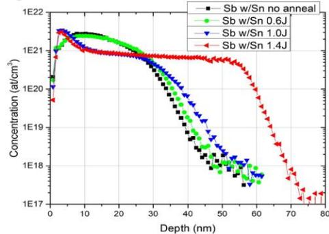
Fig.8: Sb SIMS profiles comparing Sn+Sb implant region for no anneal up to  $1.4J/cm^2$ .
