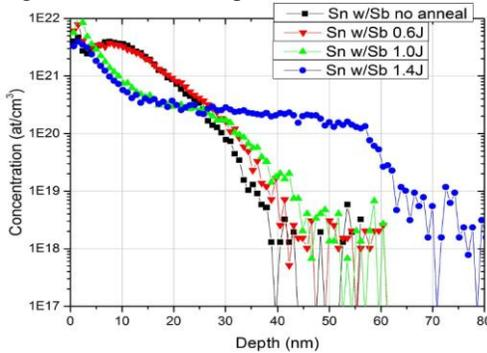
Fig.9: Sn SIMS profiles comparing Sn+Sb implant region for no anneal up to  $1.4J/cm^2$ .
