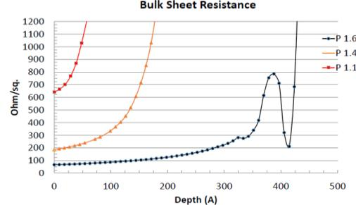
Fig.11: Differential Hall P- $R_s$  n+ depth profiles.
