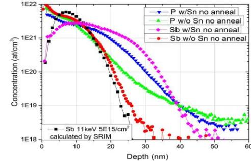
Fig.3: No anneal region SIMS profile showing channeling and non-channeling n+ profiles.
