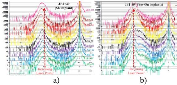
Fig.12: XRD strain-Ge analysis for a) Sb and b) Sn+P implant regions with increasing laser energy density.
