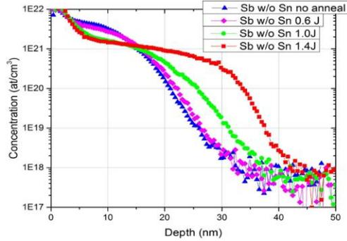
Fig.7: Sb SMS profiles for 0.0, 0.6, 1.0 and  $1.4J/cm^2$  laser anneal conditions.
