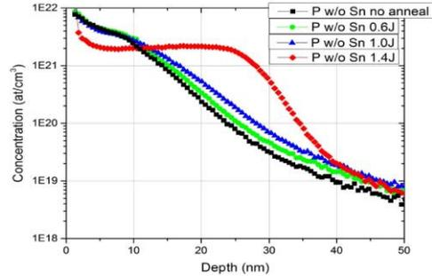
Fig.4: P SIMS profiles for 0.0, 0.6, 1.0 and 1.4J/cm<sup>2</sup> laser anneal conditions.
