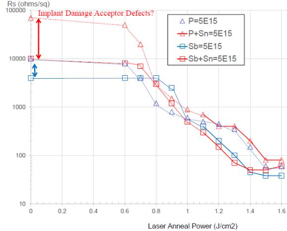
Fig.2: Hx-4PP Rs sheet resistance for various laser annealing conditions.
