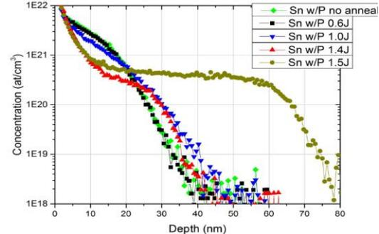
Fig.6: Sn SIMS depth profiles for the Sn+P implant region comparing no annealed up to 1.5J/cm<sup>2</sup>.
