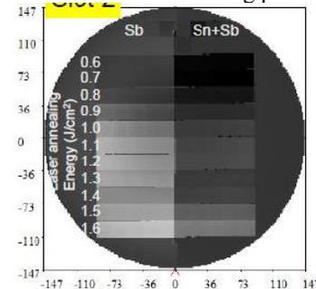
Fig.1: TW wafer map showing laser anneal regions.
