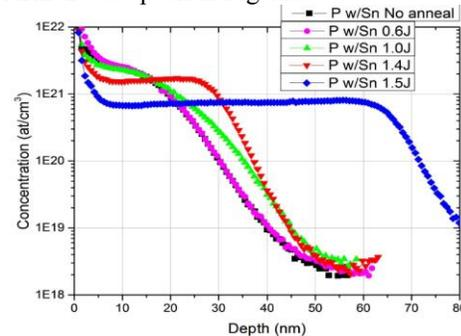
Fig.5: P SIMS for Sn+P implant region with 0.0, 0.6, 1.0, 1.4 and 1.5J/cm<sup>2</sup> laser anneal conditions.
