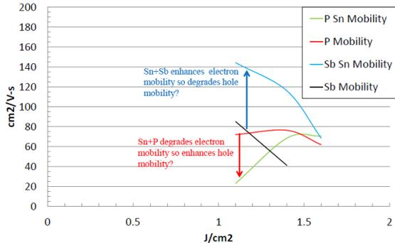
Figs.13: Electron mobility versus laser energy density.
