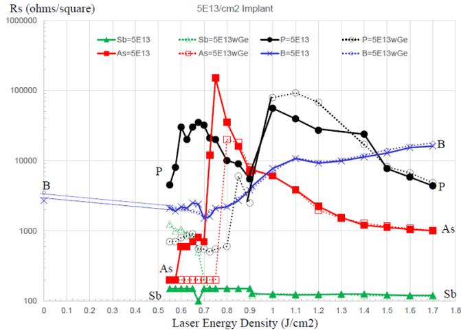
Fig.4. Hx-4PP Rs results for high and low dose P, As and Sb w/ & w/o Ge-PAI.
