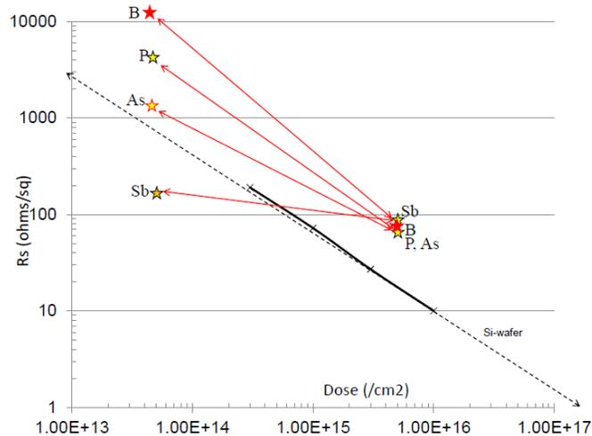
Fig.5. Rs versus implant dopant dose.
