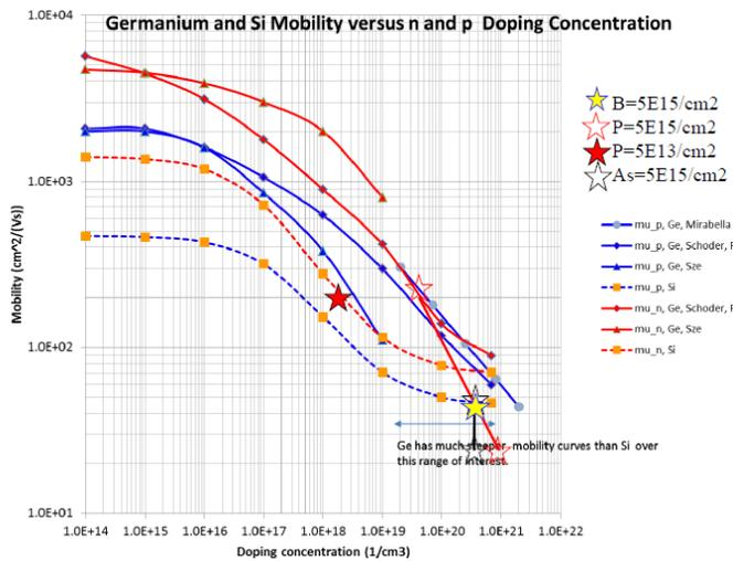
Fig.7. Comparison of Ge-epi USJ ALPro bulk drift mobility to Si and Ge reference electron and hole mobility.
