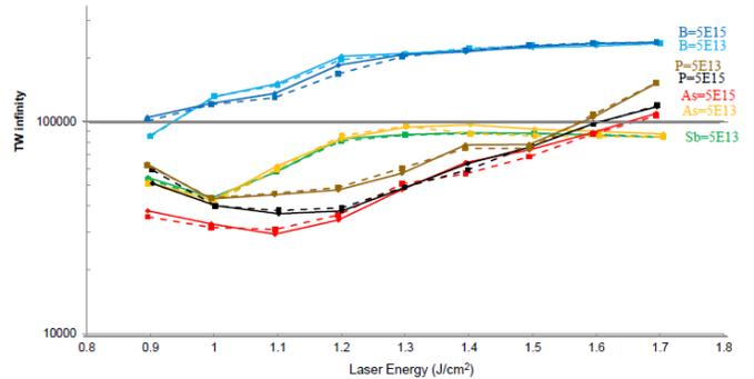
Fig.6. Ge-epi USJ implant and laser anneal damage recovery analysis by therma-probe (TW) measurement.
