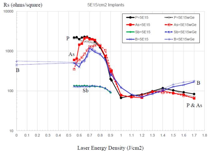
Fig.3. Hx-4PP Rs results for high and low dose B w & w/o Ge-PAI.
