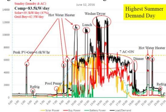
Fig.7. Off-line excel data analysis of the Laplace collected data with 1 minute resolution.
