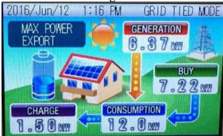
Fig.5. Tabuchi Electric remote wall solar system monitor in real-time with data refresh every 5 seconds.
