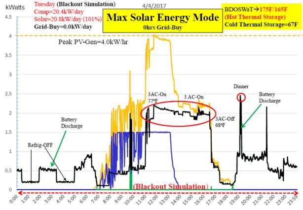
Fig. 13. Max Solar Energy mode with 3 AC units on.
