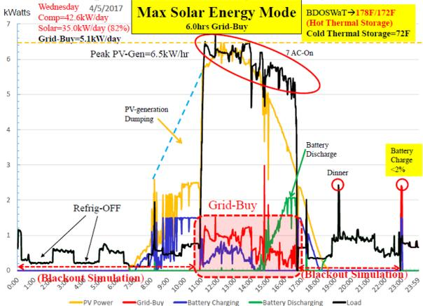
Fig. 12. Max Solar Energy mode with 7 AC units on.
