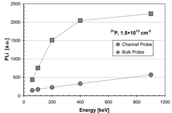
**FIGURE 3.** Impact of implantation energy on PLi levels for  $^{31}\text{P}$  specie implanted at a  $1.5 \times 10^{13}$   $\text{cm}^{-2}$  dose.
