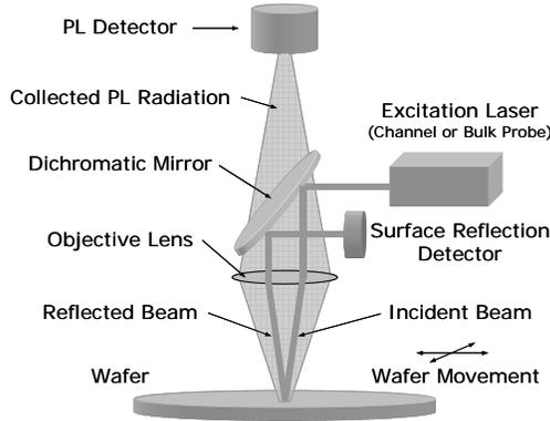
**FIGURE 1.** RTPL measurement setup.
