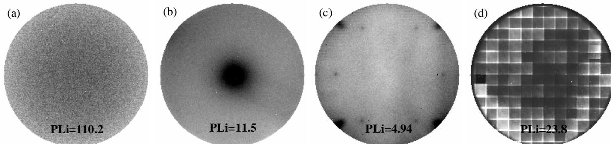
**FIGURE 7.** PL images of post-implantation annealed samples illustrating signatures of annealing equipment; (a) SPE, (b) spike, (c) flash, and (d) laser. All samples implanted with  $^{11}\text{B}$ ,  $1 \times 10^{15} \text{ cm}^{-2}$ , 500 eV (without PAI).
