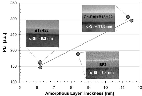
**FIGURE 5.** Correlation of PLi levels to amorphous layer thickness for USJ samples implanted at  $10^{15} \text{ cm}^{-2}$  equivalent dose. The thickness values were determined by TEM.
