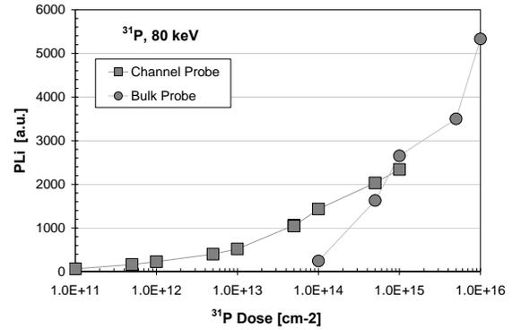
**FIGURE 2.** Impact of implantation dose on PLi levels for  $^{31}\text{P}$  specie implanted at 80 keV.
