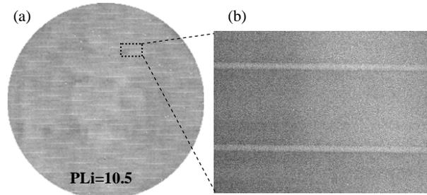
**FIGURE 6.** (a) PL full wafer map and (b) micromap showing close-up of stripping caused by overlap region.
