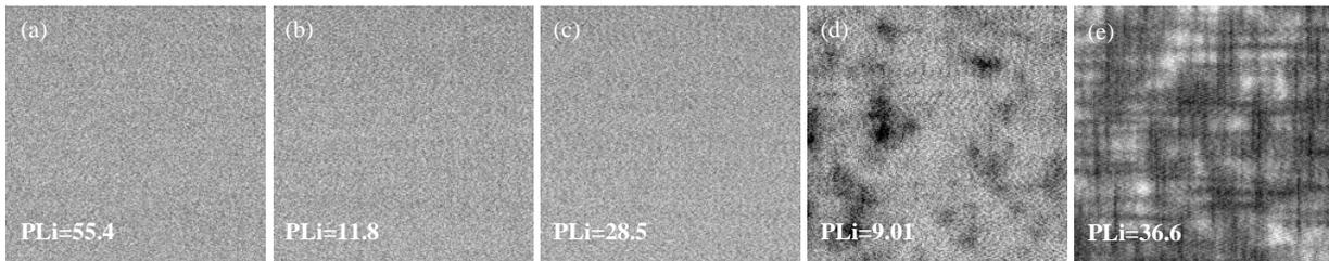
**FIGURE 8.** PL micro-images of annealed samples illustrating residual defectivity signatures of annealing process; (a) SPE, (b) spike, (c) flash I, (d) flash II, and (e) flash III;  $^{11}\text{B}$ ,  $1 \times 10^{15} \text{ cm}^{-2}$ , 500 eV, with PAI implantation;  $200 \mu\text{m} \times 200 \mu\text{m}$ ,  $1 \mu\text{m}$  step images.
