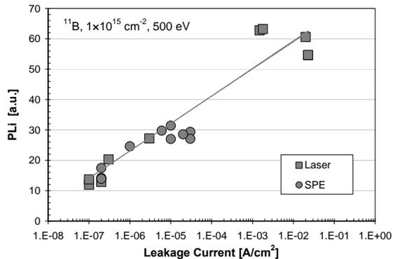
**FIGURE 9.** Correlation of junction leakage by RsL method (4) to residual defectivity by PLi.
