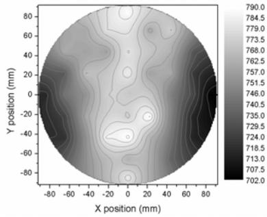
**FIGURE 4.** Ion implanter signature,  $^{31}\text{P}$ ,  $E = 60 \text{ keV}$ ,  $C_s = 1.5 \times 10^{13} \text{ cm}^{-3}$ , as-implanted sample.
