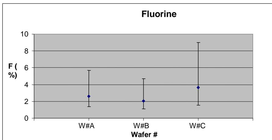
Fig. 12: XPS detected high levels of F cross contamination. Error bars reflect range of F composition
