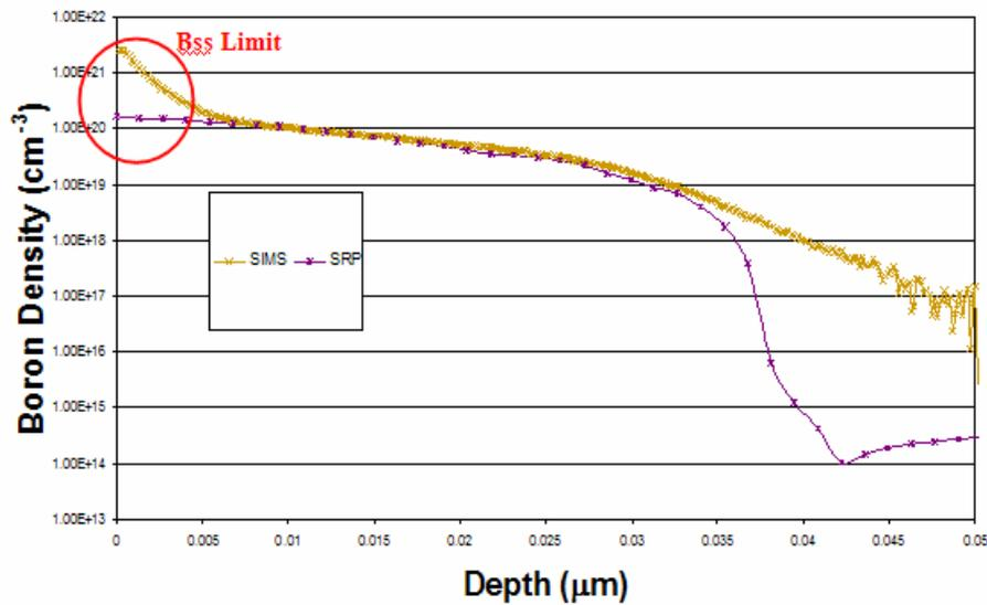
Fig. 2: Good agreement between SIMS and SRP profiles has been observed with significant diffusion (1).
