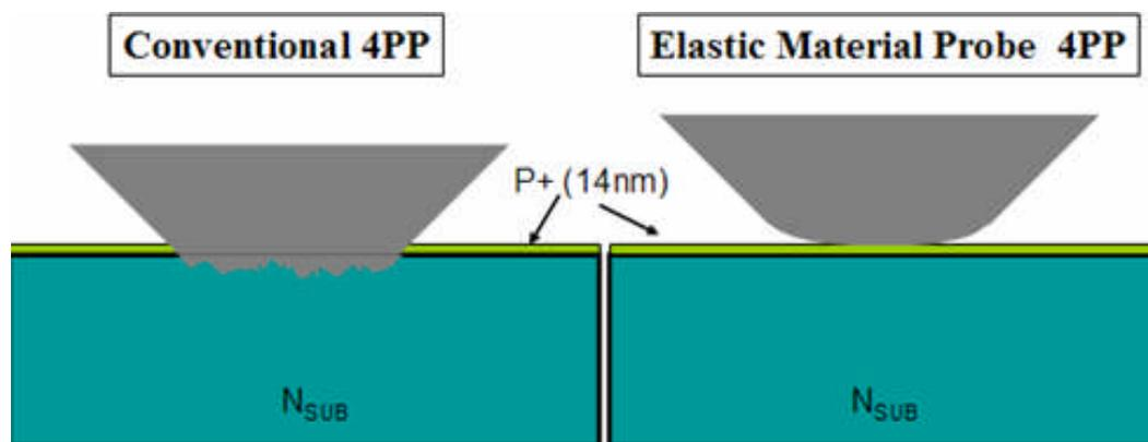
Fig. 4: Probe penetration through shallow junctions (2).
