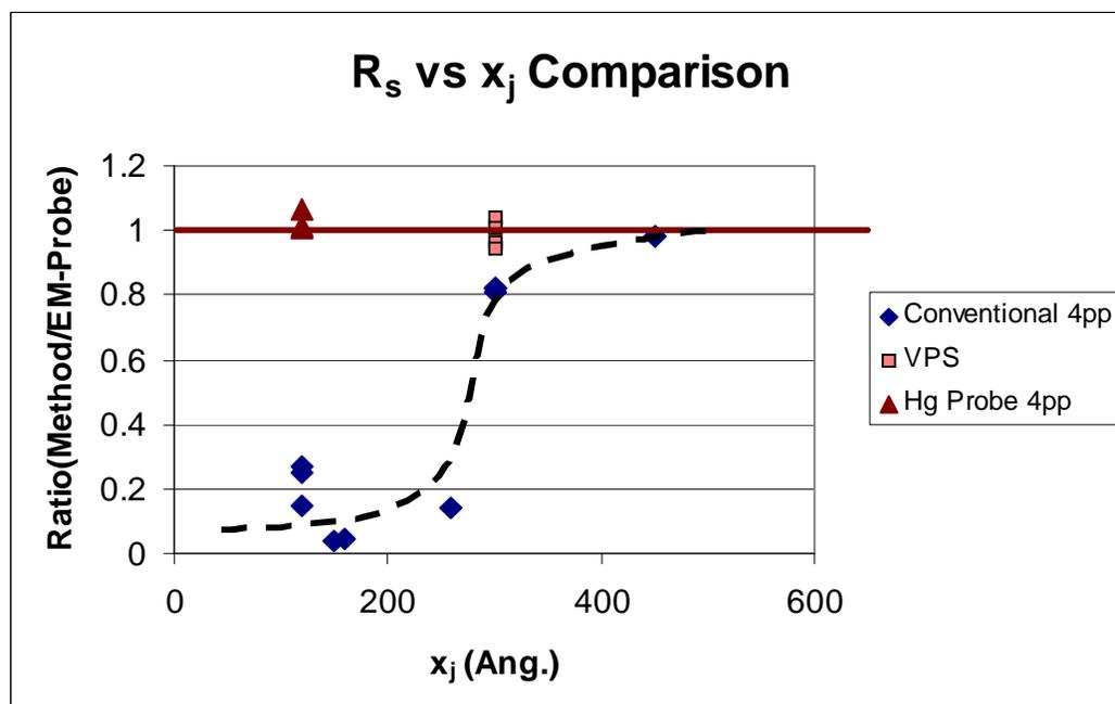
Fig. 5:  $R_s$  result comparison between penetrating and non-penetrating probes on shallow junctions from 50nm down to 14nm (2).
