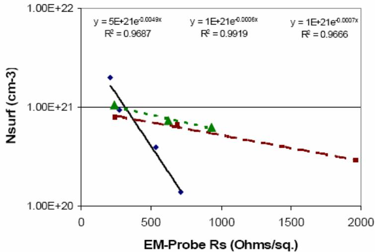
Fig. 8: Correlation plot of EM-Probe  $N_{SURF}$  versus EM-Probe 4pp  $R_s$ .
