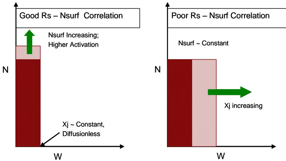
Fig. 7: Two profiles showing that either activation level or increased diffusion (deeper junction) can improve Rs measured by 4PP.
