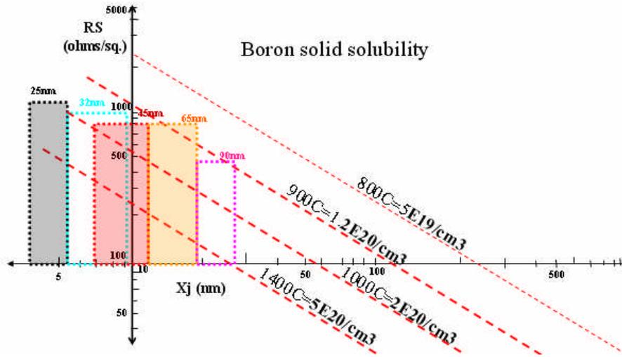
Fig. 1: Bss temperature dependence plotted as Rs versus Xj.
