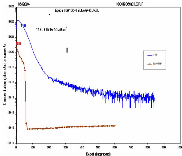
Fig. 3: Poor agreement between SIMS and SRP profile is observed with diffusion-less activation (3).
