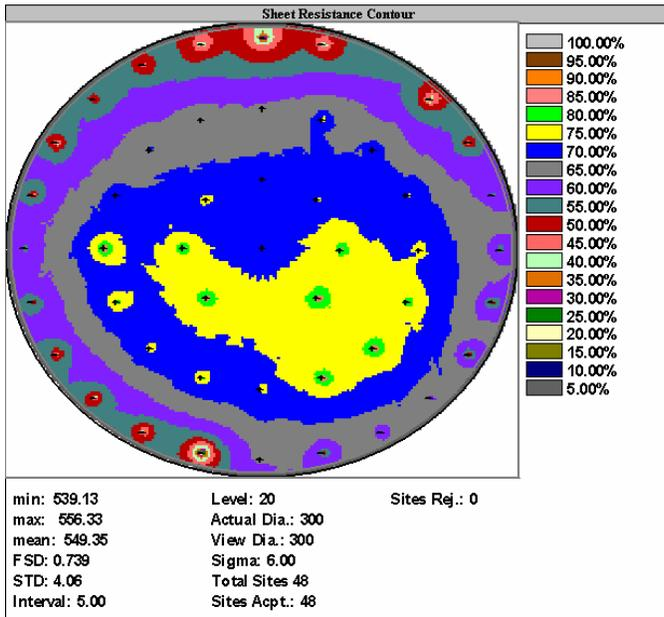
Fig. 6: 300mm wafer Rs mapping by EM-4PP.
