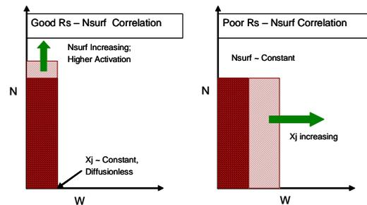
Figure 8 Two profiles showing that either activation level or increased diffusion (deeper junction) or both can be modified.
