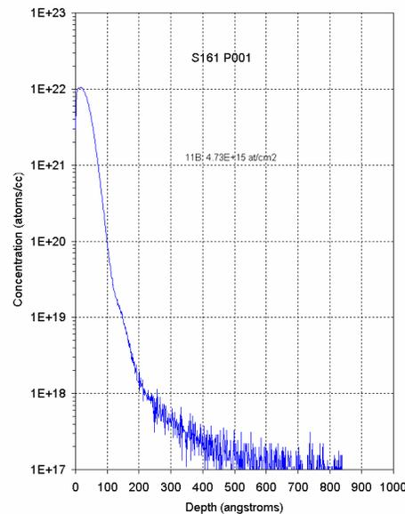
Figure 4: SIMS profile for wafer S161
