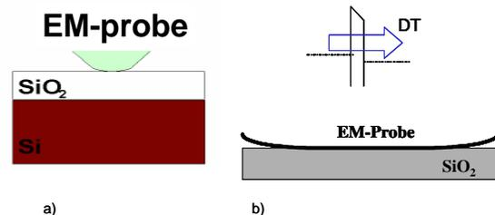
Figure 1: Schematics of an EM-Probe MOSCAP.
