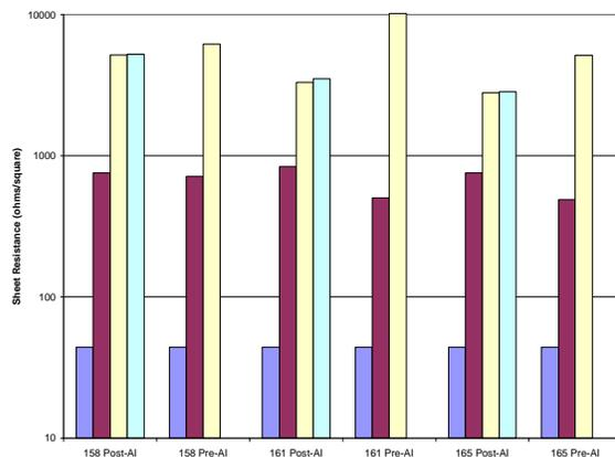
Figure 6: Sheet resistance data measured with advanced 4pp, EM-probe 4pp and Hg 4pp.
