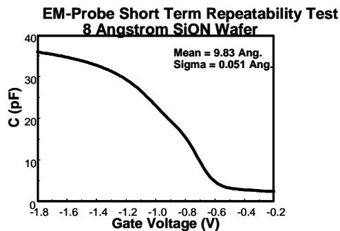
Figure 2: EM-Probe CV curve measured on an 0.8 nm oxide.
