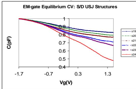
Figure 10 Normalized EM-probe CV curves obtained on the samples shown in Fig. 13. The values of N<sub>SURF</sub> are obtained from the measured maximum and minimum capacitances.
