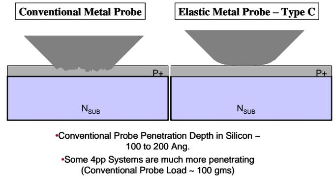
Figure 3: Another illustration pointing out the penetrating versus non-penetrating nature of the Conventional and EM-Probe 4pp designs.
