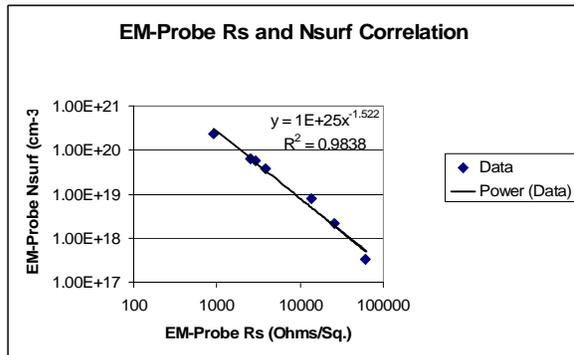
Figure 11 Correlation plot of EM-Probe N<sub>SURF</sub> versus EM-Probe 4pp R<sub>S</sub>.
