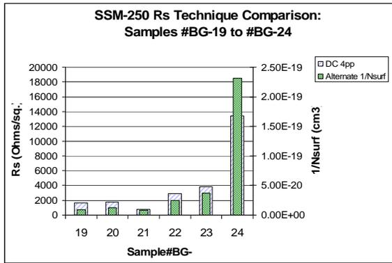
Figure 9 Histogram comparison of EM-Probe 4pp R<sub>S</sub> and EM-Probe N<sub>SURF</sub>. The measured EM-probe CV curves for the sample results shown in Figure 9 are provided in Figure 10.
