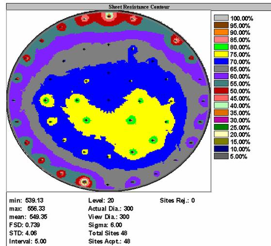
Figure 7 300 mm Wafer map of EM-Probe 4pp  $R_S$ .
