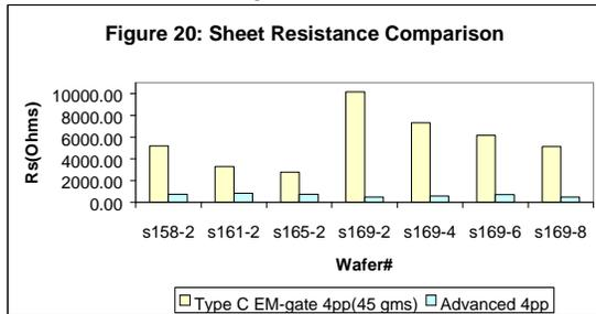
Figure 5: Sheet resistance data measured with both scrubbing and EM-probe 4pp systems.
