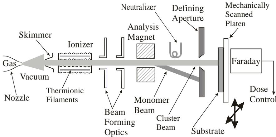
Fig. 2: Schematic of Epion's infusion doping equipment.
