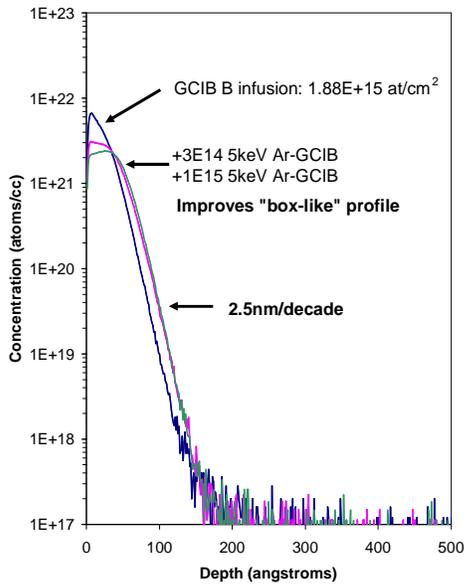
Fig. 8: Transient thermal spike localized heating effects creating a more box-like shaped boron profile.
