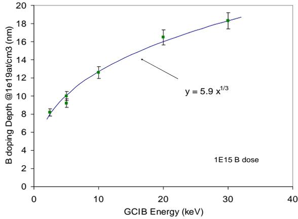
Fig. 7: Junction depth to the 1/3 power for infusion B doping.
