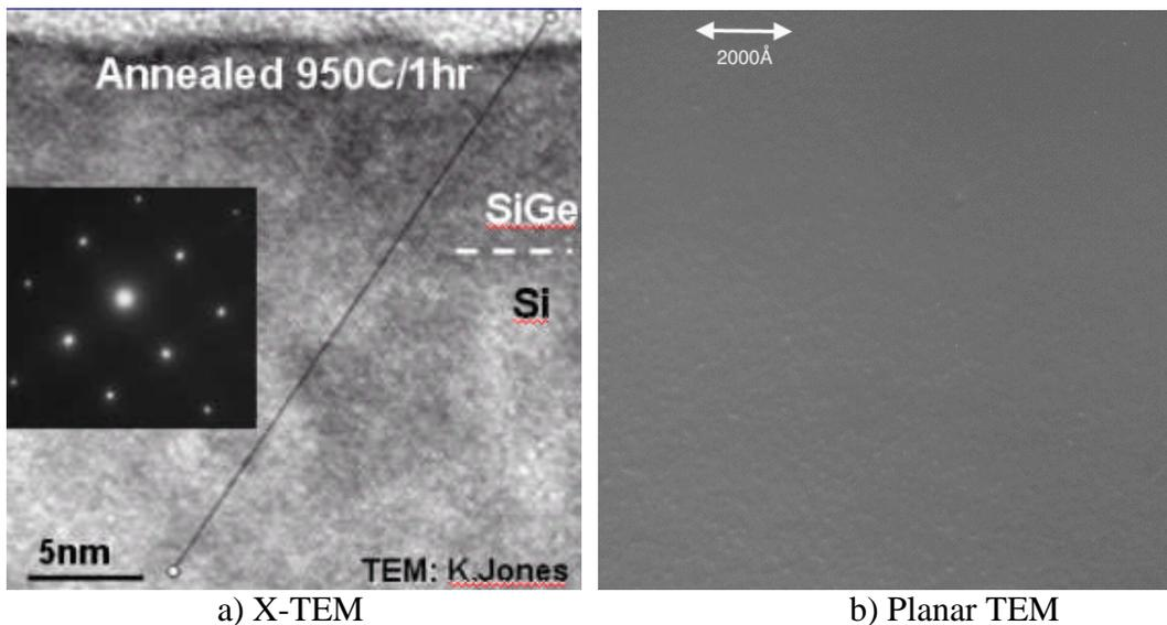
Fig. 16: 12nm Ge infusion doping/deposition after 950°C anneal showing defect free single crystal SiGe layer after 950°C 1 hour anneal a) X-TEM free of defects and b) defect free planar TEM.
