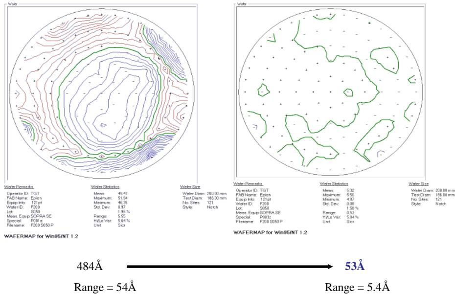
Fig. 4: Localized GCIB corrective etching of silicon to realize uniform very thin SOI wafers.
