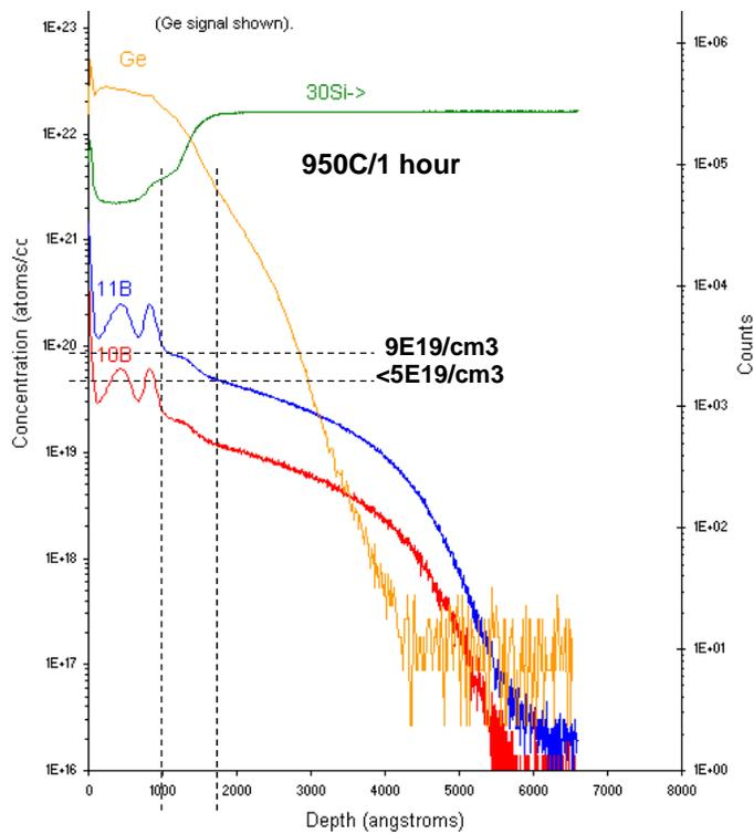
Fig. 23: SIMS analysis for 950°C annealing showing Bss increase to 9E19/cm<sup>2</sup>.
