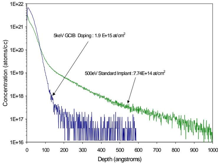
Fig. 5: SIMS comparison of implantation (channeling) and infusion (non-channeling) doping profiles of boron.
