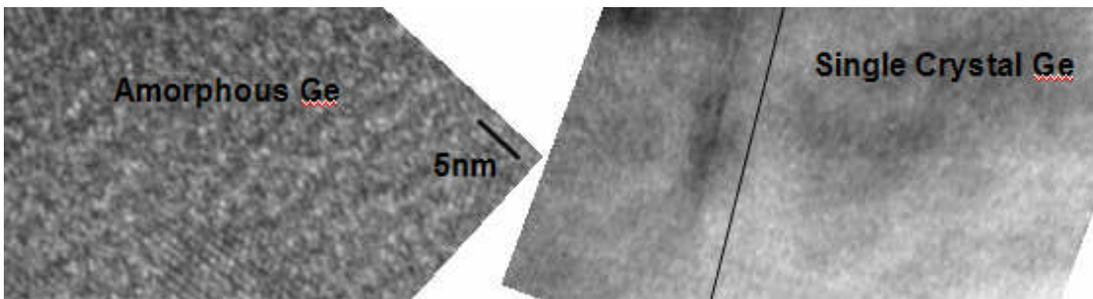
Fig. 22: Atomic resolution X-TEM showing room temp. amorphous Ge and 950°C single crystal Ge layers.
