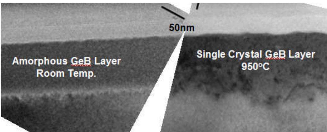
Fig. 20: X-TEM Ge infusion deposition of 90nm.
