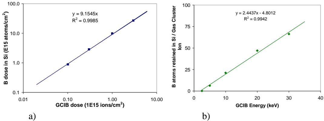
Fig. 9: Comparison between a) GCIB B dose versus silicon B retained dose and b) B doping efficiency versus energy.
