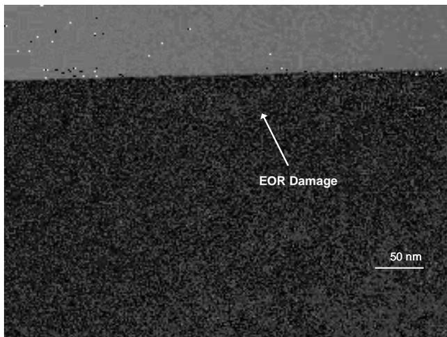
Fig. 14: 550°C annealed SPE recrystallized Ge-PAI structure with residual EOR damage (12).
