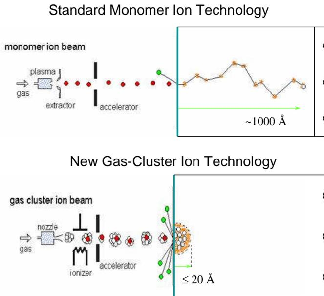
Fig. 3: Illustration comparison of monomer ion implantation versus cluster ion infusion effects.
