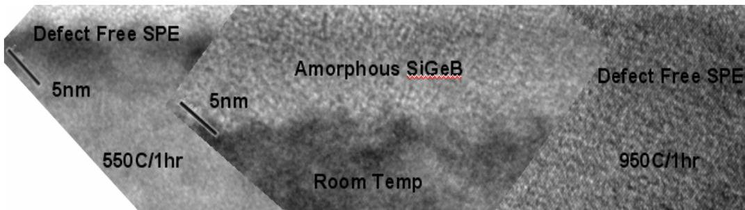
Fig. 13: Atomic resolution imaging of Fig. 8 showing defect free SPE Ge infusion layer.
