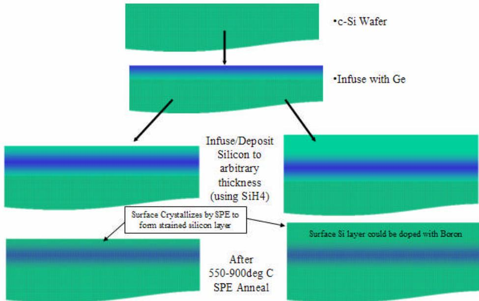
Fig. 25: DCD of 100% Ge with a Si-capping layer.
