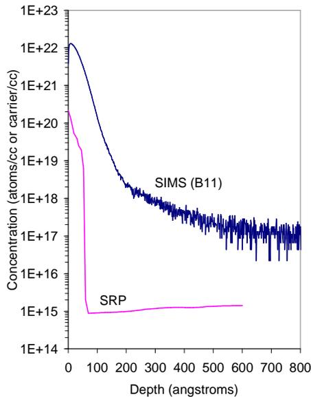
Fig. 11: Comparison of SIMS to SRP boron dopant profile (chemical –vs- electrical).
