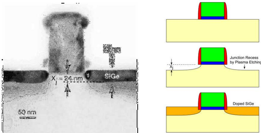
Fig. 1: SiGeB SEG for pMOS extension and raised source drain structure (1).
