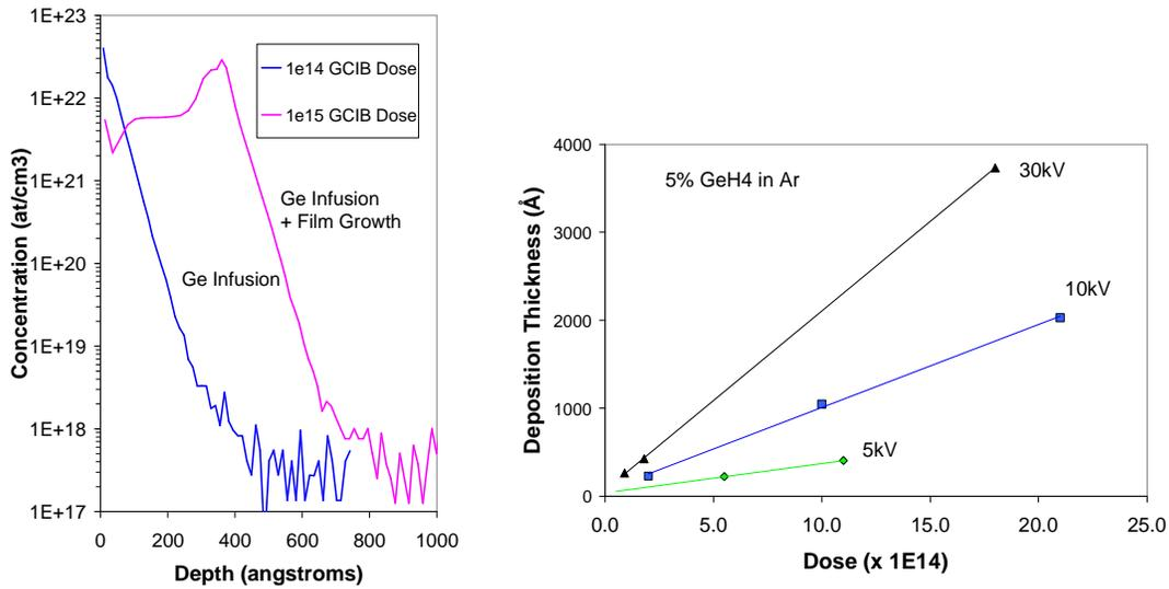
Fig. 15: Ge infusion processing; a) Ge infusion doping ( $1E14/cm^2$ ) and dose controlled deposition ( $1E15/cm^2$ ), b) comparison of 5keV, 10keV and 30keV DCD.
