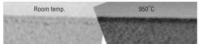
Figure 8. X-TEM of an 11-monolayer ( $1.4\text{E}16/\text{cm}^2$ ) Ge infusion deposition structure with thickness = 3.3nm.
