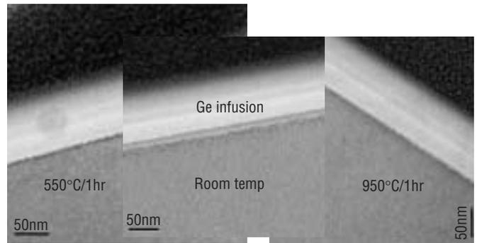
Figure 7. X-TEM of a Ge infusion doping structure to a depth of 12nm.
