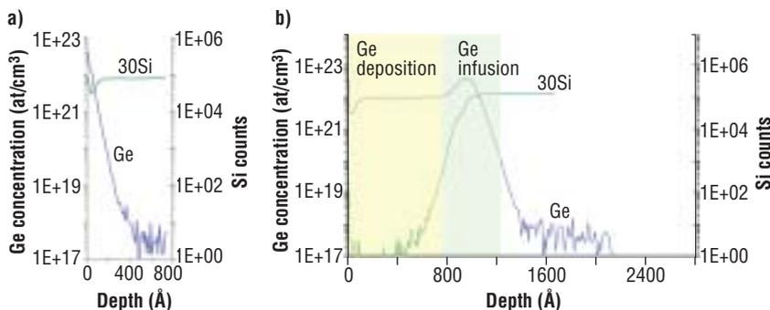
**Figure 5.** Infusion processing with a) Ge infusion doping to a depth of 34nm and b) Ge infusion deposition to a thickness of 90nm.
