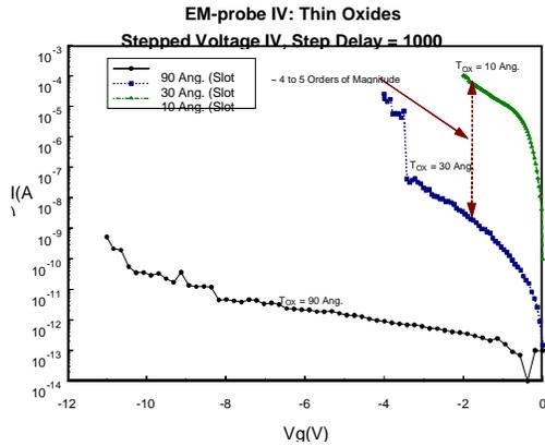
Figure 2: EM-probe IV curves measured on thin oxides with a Type C probe
