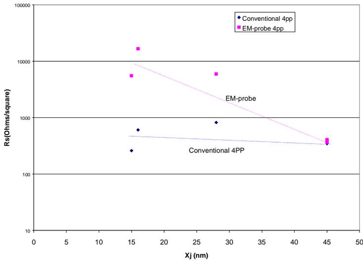
Figure 4 EM-probe and Conventional 4PP  $R_S$  comparison for samples annealed at 550 °C
