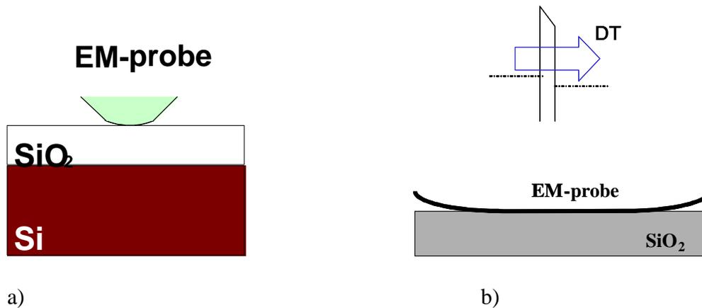
Figure 1 Illustrations of EM-probe Contact to the surface of a dielectric material.
