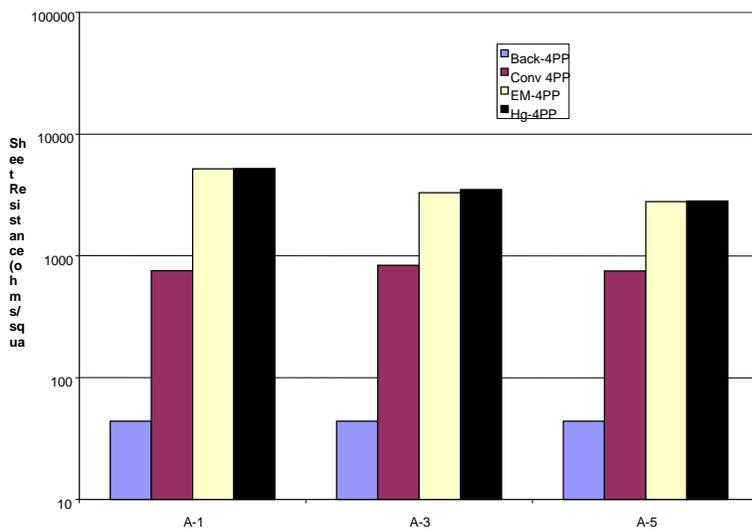
Figure 6 Comparison between 4PP, EM-probe 4PP, and Hg 4PP.
