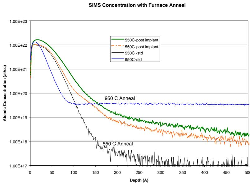
Figure 5 SIMS profiles for representative samples
