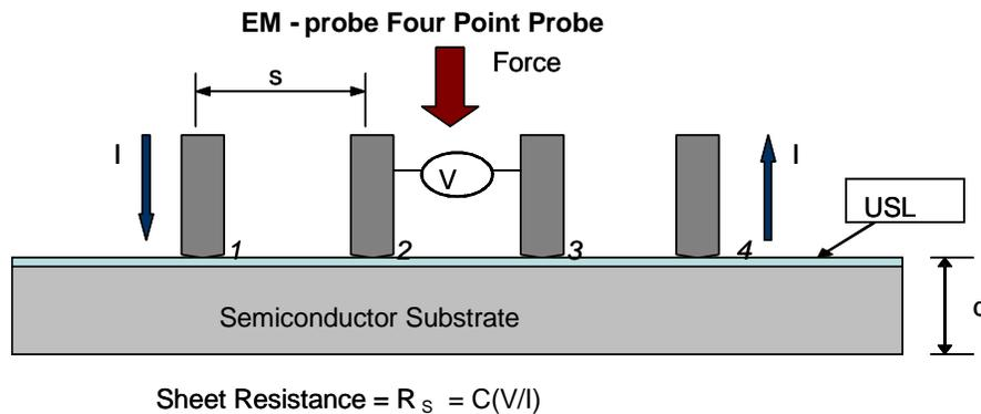
Figure 3 Depiction of an EM-probe 4PP measurement setup. The probes form a circular contact by elastic deformation and are non-penetrating and non-damaging.
