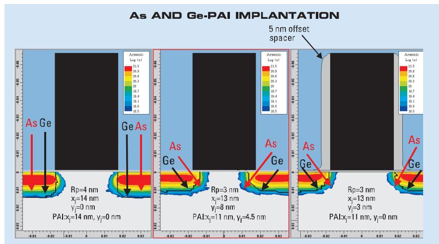
Taurus Monte Carlo implant simulation comparison of 0° tilt (left) vs. 30° quad-mode implant for As 3 keV/ $1 \sim 10^{15}$  and Ge-PAI for gate overlap control and optimization of lateral dopant profile when using diffusionless activation (center). With the 5 nm sidewall offset spacer,  $y_j$  was reduced to 3 nm (right).
