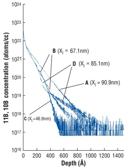
Figure 8. SIMS depth profile after SPE for plasma implanted  $\text{BF}_3$  at 5kV/2E16/cm<sup>2</sup>.
