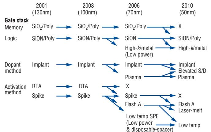
**Figure 1.** USJ roadmap alternatives based on gate stack structure.
