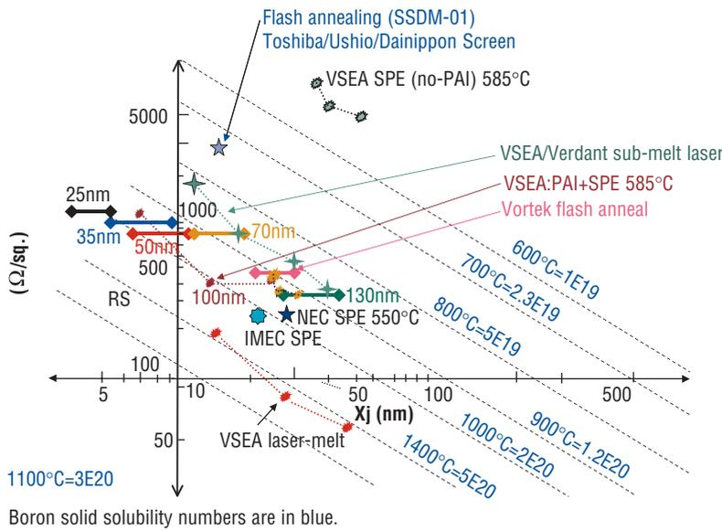
Figure 2. R<sub>s</sub> vs. X<sub>j</sub> for various activation methods.
