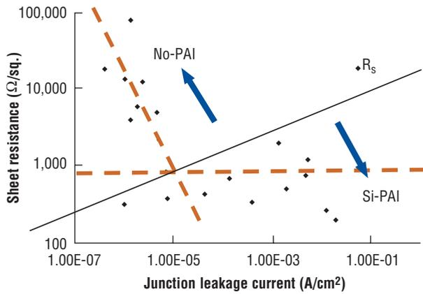
Figure 5. Low temperature SPE results for  $R_s$  vs. junction leakage.
