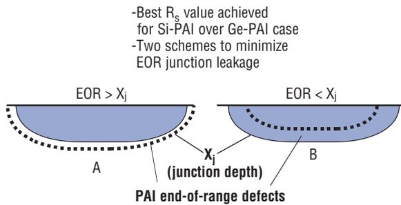
Figure 6. SPE leakage study for optimization of  $X_j$  and PAI-EOR. Scheme A is preferred if the entire transistor formed within EOR. Scheme B is preferred if S/D, S/D ext, channel formed separately. Agere characterizing diode devices on both schemes. The University of Florida is doing TEM analysis; others will also test device leakage.
