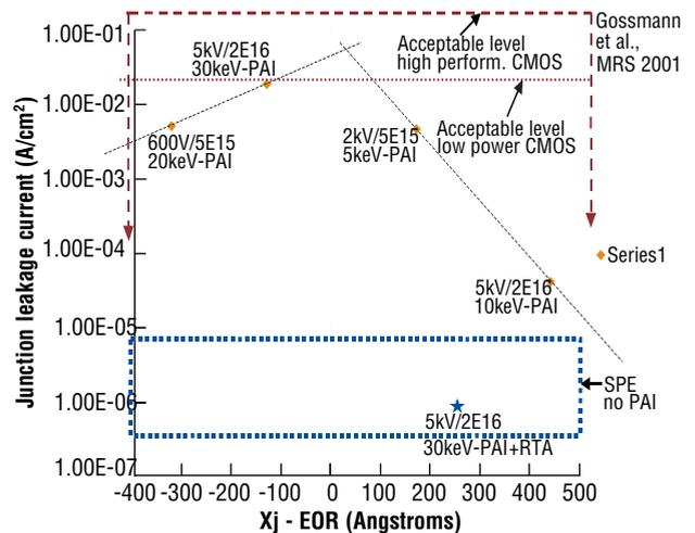
Figure 7. SPE junction leakage results for  $X_j$  and PAI-EOR optimization.
