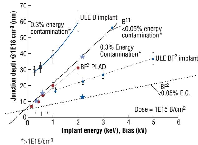
Figure 3. Boron as-implanted junction depth vs. implant energy defined at 1E18/cm<sup>3</sup>.
