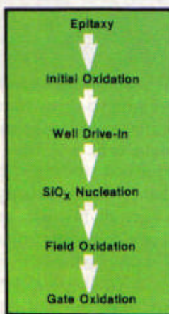
Fig. 15—CMOS process flow to achieve enhanced-process induced gettering.
